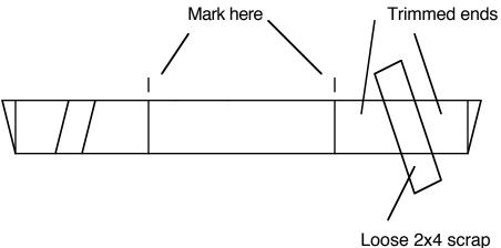
Place a scrap 2"x4" next to it just as a place holder and add the other non trimmed end piece. Glue and screw these down to create a slot the 2"x4" can slide through on each end. These will eventually form the mortis that the legs slide into.
