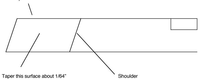
Taper out to the end from the shoulder this will allow the tenon to slide in easily abut make a firm joint when in all the way.
