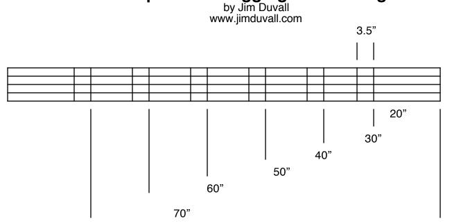
Set your circular saw blade to a depth of 1.25" and cut along the lines creating dadoes 3.5" wide that will fit a 2"x4" snugly. A snug fit here is important.
