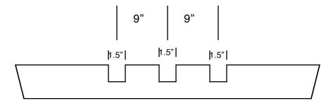
Set your circular saw to make a 3.5" deep cut and cut slots in the tops of both boards as they are clamped together. Make repeated cuts until material is removed so that a 2"x6" will slide into each slot firmly. Clean up with a sharp wood chisel. Take care to make slot firm but wide enough so that board will slide in to bottom. These will be your inside rail pieces.
