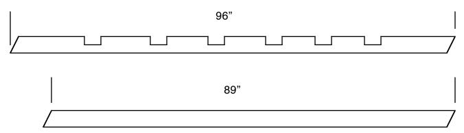
Now line up the inner and outer legs apply construction adhesive and screw them together. Be sure to create a left and right leg for each end of the rack.
